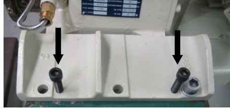
Figure 3-3: illustrates adjustment screws for length & lateral adjustment.
